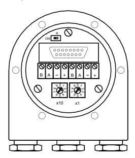
The Profibus-DP device address is set by user-friendly rotary switches in the connection cap. Allowed addresses are between 1 and 99, each can only be used once. The connection cap can be opened for installation by removing the six cap screws.
