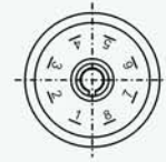
Terminal Wiring (Top View)
