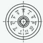
Terminal Wiring (Top View)
